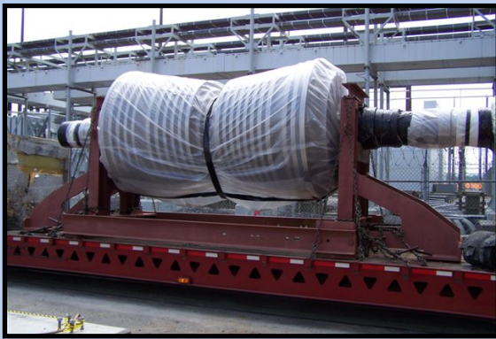
High Pressure Turbine for Unit 2 being delivered
